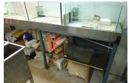
Stainless Steel Bench with Drain 2290 mm x 405 mm wide x 35 mm deep inside 105 mm Outside c/w Steel
